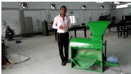
Assembled Power Operated Maize Sheller
