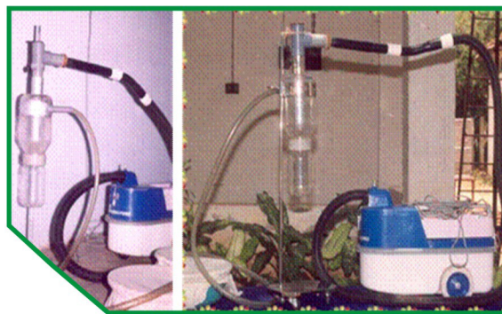
TNAU Corcyra moth collector with minimum health hazard
